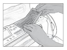
Place the keypad overlay on top of the machine's keypad.
