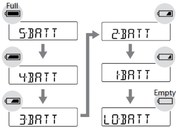
After the "LO-BATT" alert flashes for 8 seconds, the unit will turn off automatically.
