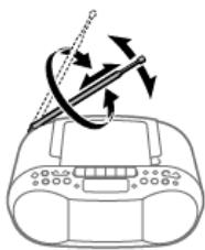
Extend the telescopic antenna **⑦** and adjust its length and angle for optimum reception.
