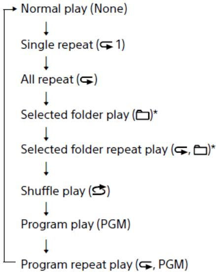
\* These functions are available only when playing MP3 files on an MP3 disc.
