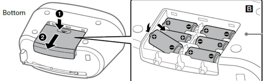
Press down on the battery compartment cover at **1** and slide it in the direction of the arrow **2**.
