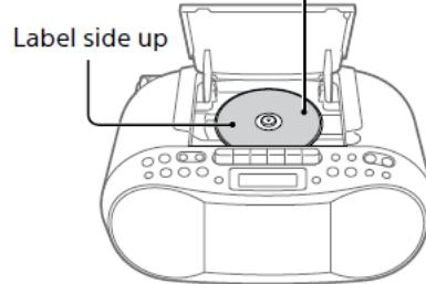
The disc is loaded and the disc information appears on the display.
