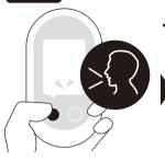
Speak into the device while holding down the button. Let go of the button to translate.
