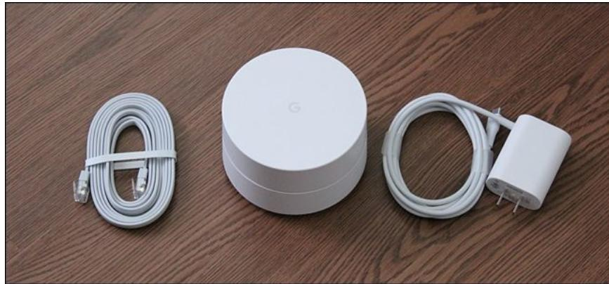
Next, plug in the first Google WiFi unit into an outlet and connect the other end into the USB-C port on the bottom of the unit. Then take the ethernet cable and plug one end into the ethernet port on your modem and the other end into the green ethernet port on the Google WiFi unit. If you have a modem/router combo, simply just plug the ethernet cable into any one of the numbered ethernet ports on the combo unit.
