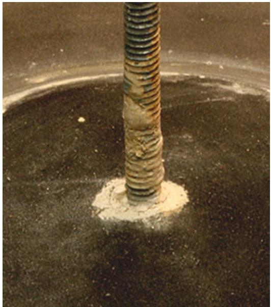
This picture is of a rusty center rod with caked-on grit slurry. It's likely that moisture has gotten under the foam pad and started to rust the base plate.
