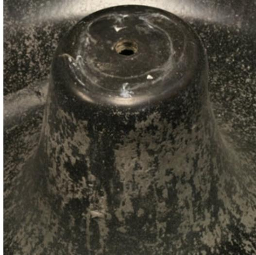
The gray material that you see in this barrel is dried rock mud. If this is not completely cleaned off, it will contaminate the next step of the tumbling process, and your rocks will not achieve their brightest possible shine.
