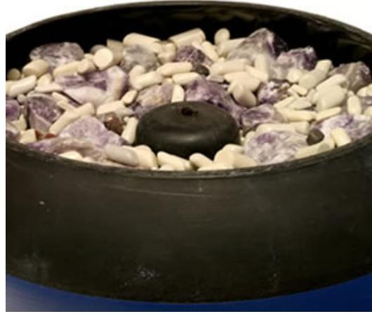
This photo shows a properly filled UV-10 tumbler bowl. Notice the level of material is just below the top of the bowl's center structure.
