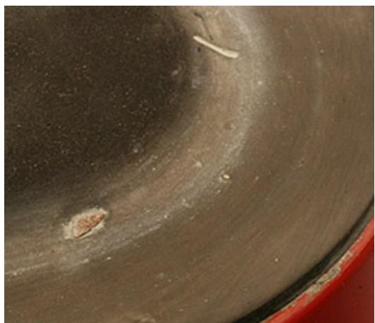
Debris on the base pad can wear a hole in the bowl or the pad if not removed.
