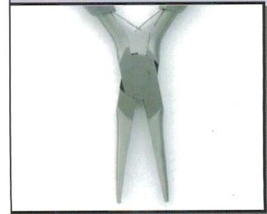
**Flush-cutters** allow a flat, even cut when trimming headpins, eye pins, or beading wire. This tool is easily ruined if used on memory wire. Please take precautions.
