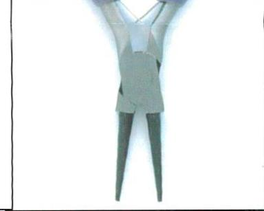
**Flat-nose pliers** are used to bend wire and hold beads when needed. The flat inside surface of the jaws help open and close jump rings, flatten wire or to hold a wire in place while wrapping. These give you stability when working with different components.
