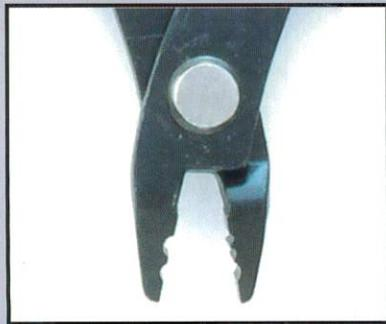
**Chain-nose pliers** are very versatile and used for a variety of different applications. They are used to reach tight places, close jump rings, bend wire and stabilize a design while working. They are great for picking up small beads and findings. They become the extra fingers for a jeweler.
