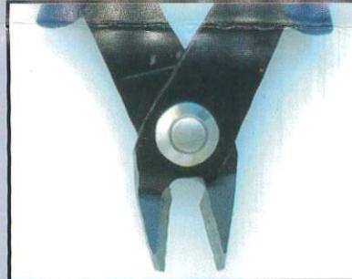
**Round-nose pliers** are an invaluable tool when working with wire. They are used to create loops and curls on the wire. They are also extremely helpful when making drops or earrings. They assist in making the loops in pins.
