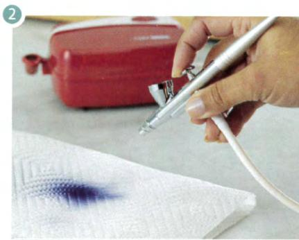
**Keep it Clean:** It is very important to clean the airbrush between color changes and at the end of each use to keep it working properly. Never allow color to dry inside the airbrush. See pages eight and nine of this guide for complete instructions on cleaning your airbrush.
