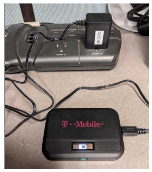
To turn off the hotspot simply press the power button for 3 seconds. A "goodbye" message will appear on the display screen.
